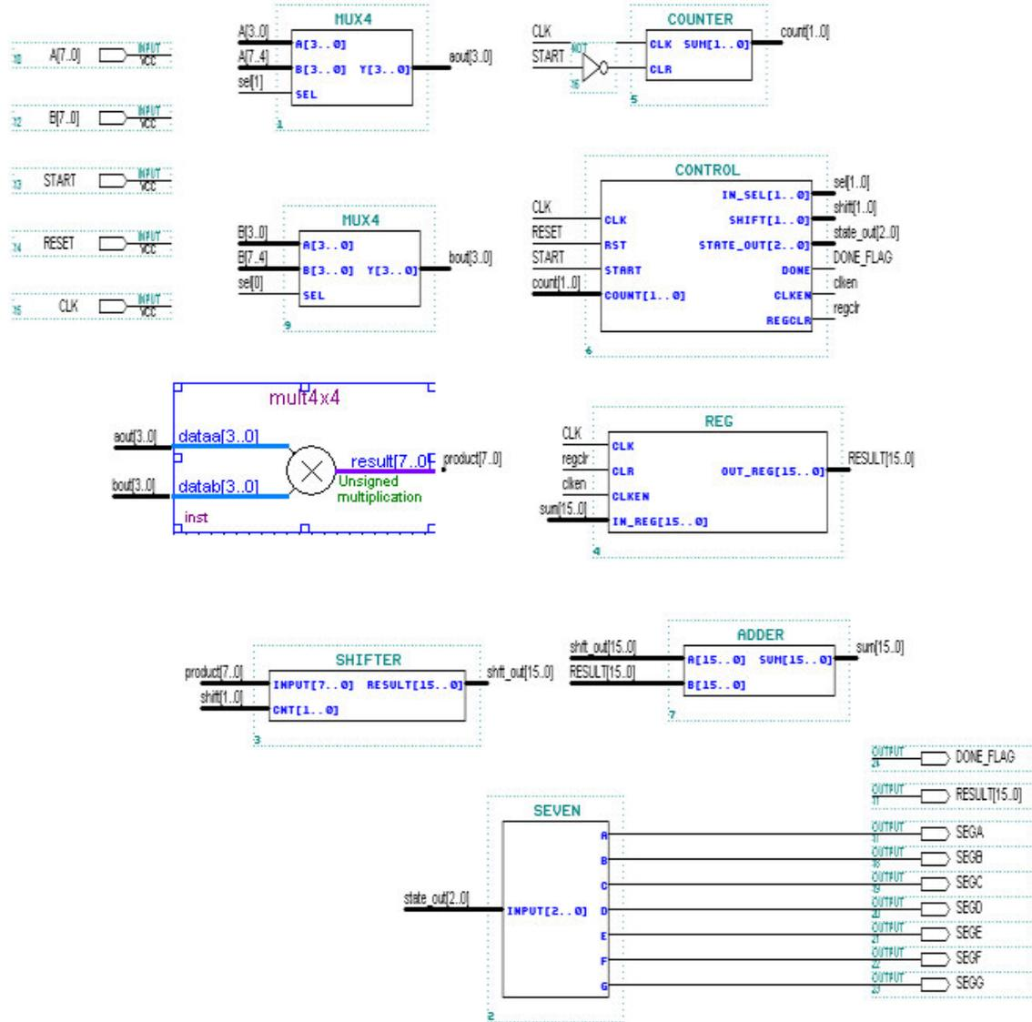
Figure 1 - 8 X 8 multiplier top level design block diagram
