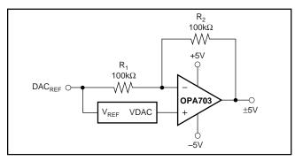
FIGURE 10. Bipolar Operation with the DAC.
