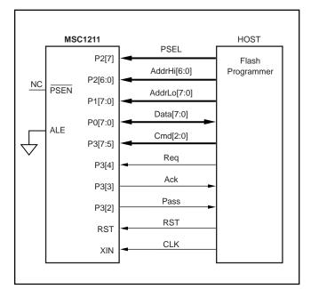
FIGURE 14. Parallel Programming Configuration.
