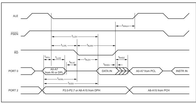
FIGURE B. External Data Memory Read Cycle.
