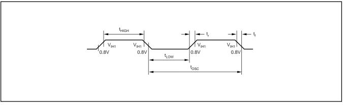
FIGURE D. External Clock Drive CLK.
