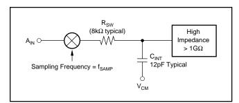
FIGURE 6. Analog Input Structure.
