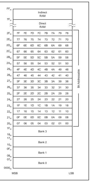
FIGURE 13. Scratchpad Register Addressing.
