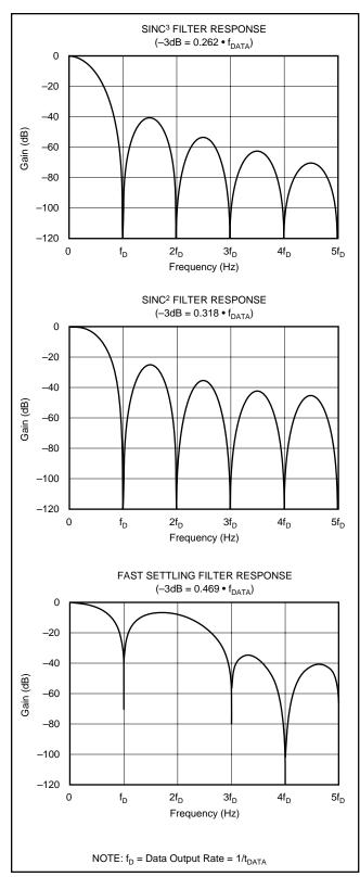
FIGURE 8. Filter Frequency Responses.
