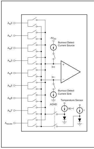
FIGURE 5. Input Multiplexer Configuration.
