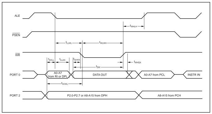
FIGURE C. External Data Memory Write Cycle.
